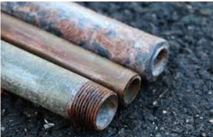
(L-R) Galvanized, Copper, Lead Pipe
