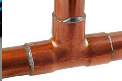
Copper w/Lead Solder
